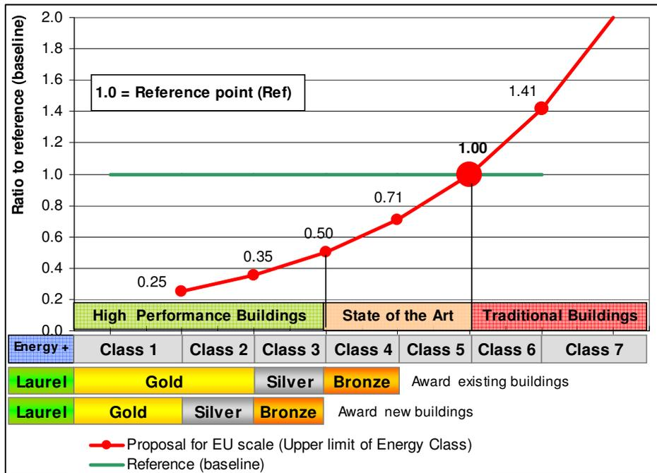
Figure 4: Limits of proposed energy classes (ratio real/ reference)
