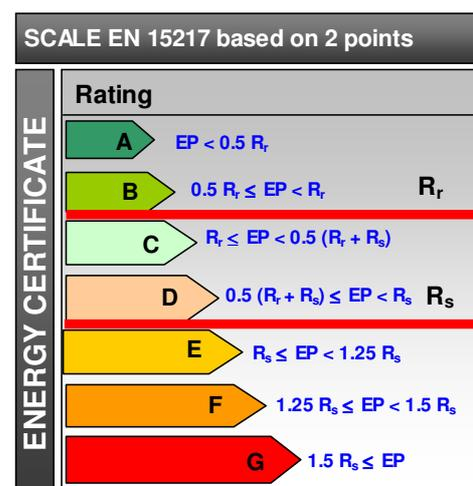
Figure 1: Scale based on EN 15217.
