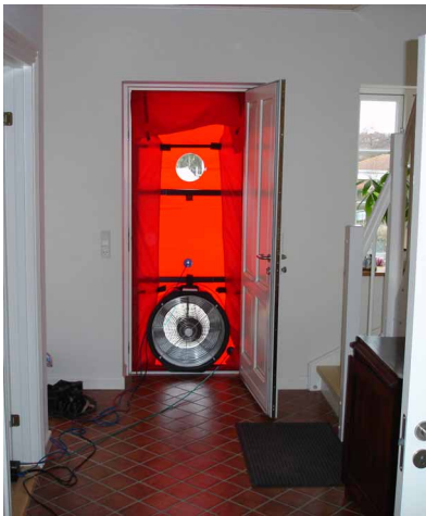
Air tightness proven by Blower Door test
