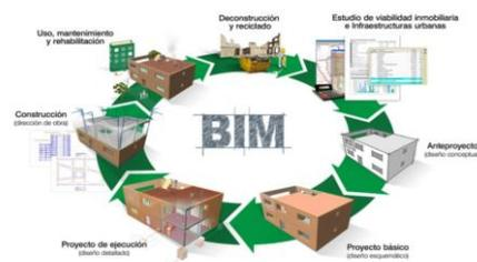
involved in the different construction processes. Working with BIM (building information modelling) implies using a single model to generate and manage all the project information throughout its entire life cycle.
